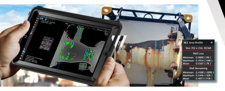
Doppler Z-MLE is VMI's game-changing, patented tool for pipe wall-loss measurement beyond traditional tangential radiography. Inspectors can now access more comprehensive wall-loss information across the entire radiograph. This provides data to foster optimized decision making and faster fit-for-service calculations.
